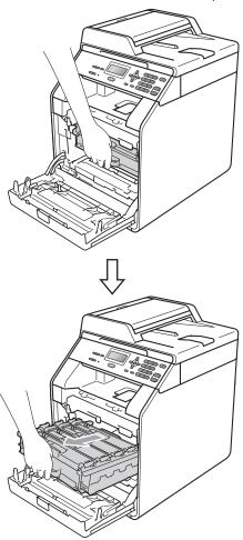
4 Turn the green lock lever (1) at the left of the machine anticlockwise to the release position. Holding the green handles of the drum unit, lift the front of the drum unit and remove it from the machine.
